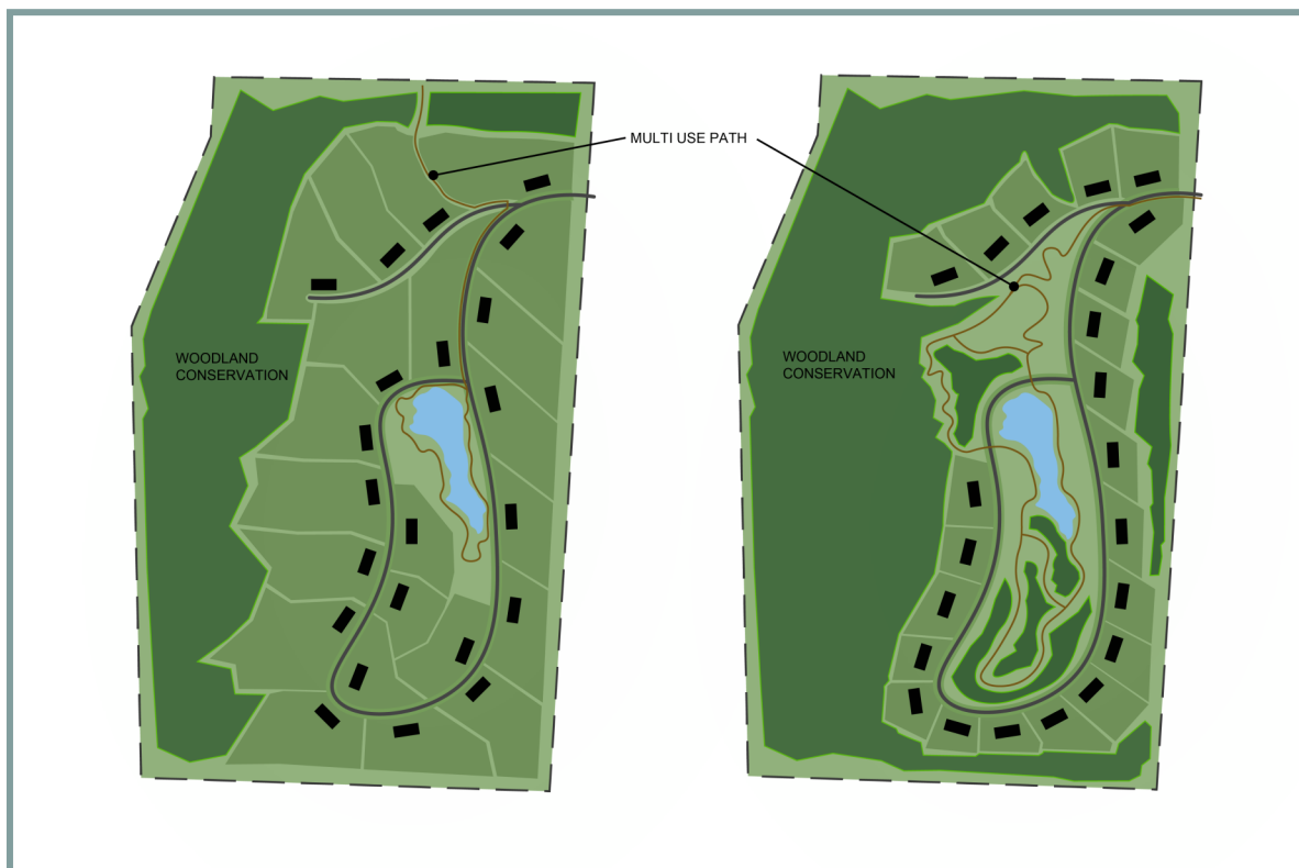
Figure 45: Conceptual renderings of clustered conservation housing, where the left tract highlights an example of on-site septic systems, and the right image displays a layout where central water and sewer are utilized.
